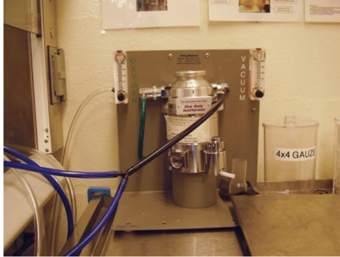
Figure 15G.2.3 Induction chamber in the BSC is connected to an isoflurane vaporizer through tubing.
